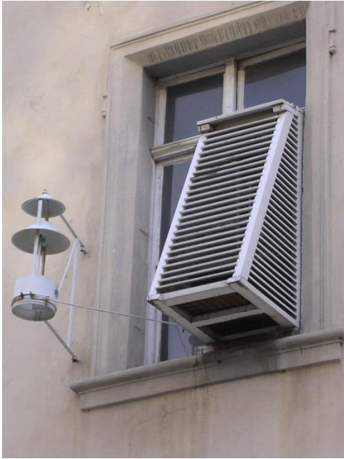
Fig. 4 Detail of the placement of the thermometers at the station in Prague Klementinum
