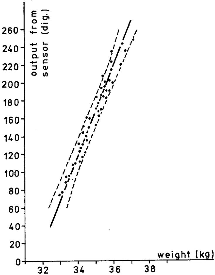
Figure 2. Output of VIRRIB versus the weight of the soil block.
